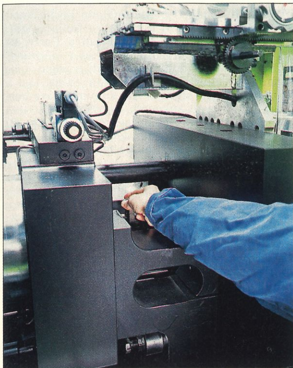
FlexLink on Engel machine facilitates access to ejectors, and is easier to maintain than previous pivoting link.
